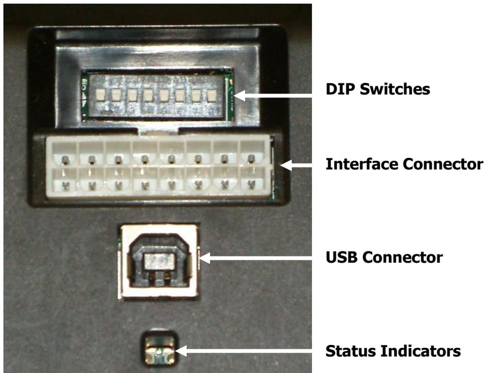
The SMART Payout unit must be powered up for the interface to be recognised by Windows. If the SMART Payout unit is not in the host machine, you will need to provide power to the 16 way interface connector first. The connection information and pin numbering is as follows:
